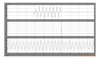
Figure13: (a)1-phase Current through TCR (b) 1-phase Current through the Capacitor (c) Line current
